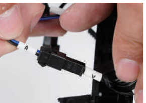
A(2PIN)→ Laser Signal Cable
