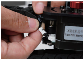
X(4PIN)→X-axis Stepper Motor Cable
