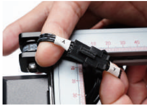
Y(4PIN)→Y-axis Stepper Motor Cable
