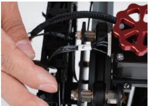
Z(4PIN)→Z-axis Stepper Motor Cable
