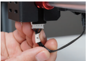
Y(4PIN)→Y-axis Stepper Motor Cable
