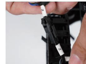
Z(2PIN)→Z-axis Endstop Switch Cable
