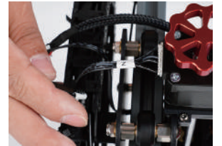
Z(4PIN)→Z-axis Stepper Motor Cable
