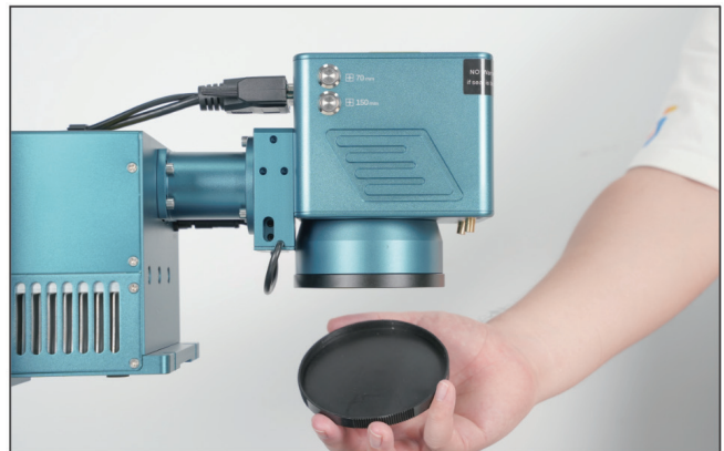
4. Remove the lens protection cover. Place the material on the baseplate, and adjust the engraving position according to the corresponding lens.
