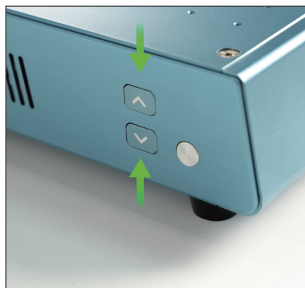
6. Hold the lifting button until the two light spots overlap. At this point, you can install the software and prepare for engraving.
