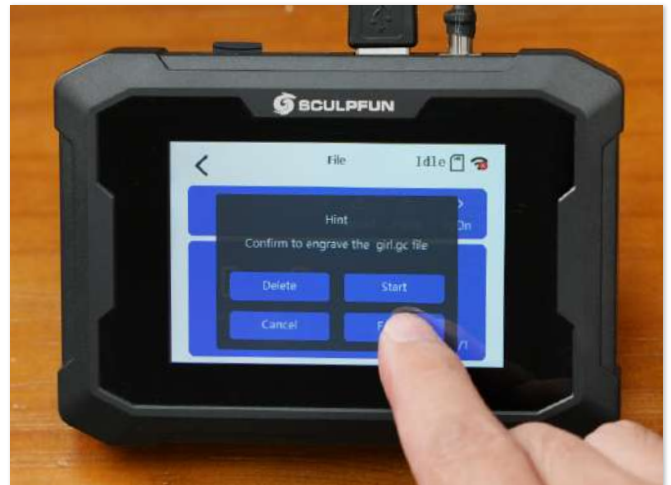
10. Select the file to be engraved and click "Frame" to ensure that the engraving range is in the appropriate position.
