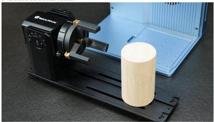
2. Secure the material in the chuck, ensuring it won't fall off. Afterward, place the roller accessory on the machine working platform. Use the mini level to adjust the level of the material for accurate printing of the pattern onto the material.
