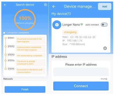
3) After the connection is successful, return to LaserBurn, select Set STA mode to connect WIFI of router (only supports 2.4G), and enter the password. The indicator light in front of Nano Pro will switch to orange breathing light during connecting, then will turn green if the connection is successful, then click the app to enter the
