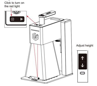
Note: The red dot is not the engraving center point, it is only used for focus reference.
