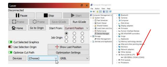
For MacOS, please go to About this Mac > Overview > System Report, select USB under Hardware, there will be USB Serial if the driver is installed automatically, and select cu.wchusbserial14230 port in the LightBurn by clicking where you see '(Choose)' in the Laser Window.
