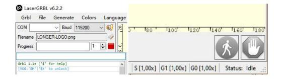
If no ports are listed in the drop-down, it means that no engravers were found, which could mean that it is not plugged in correctly, isn't powered, or the PC is missing a driver. Please click Tools menu to Install CH340 Driver from LaserGRBL software.
