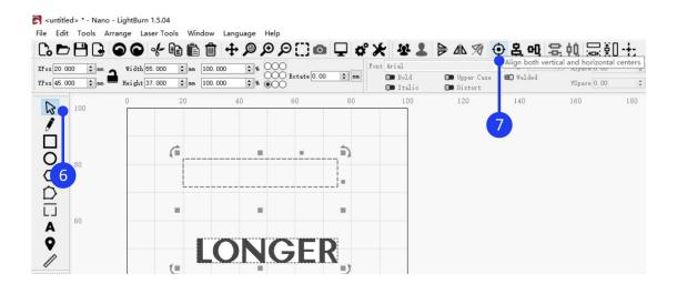
Set the coordinate point at the center of the image and enter the XY position coordinates as 50, 50 respectively, so the design is moved to the center of working size.
