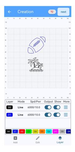
Different colored layers can set different parameters for designs to meet the needs of engraving or cutting multiple files at the same time. Such as layer mode, laser type, processing method, material, laser power, speed, times and accuracy. Up to 11 parameters can be set in the APP, first select the design to set parameters, click Layer, and select different colored layers.
