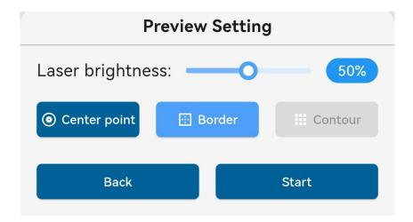
6) After confirming that the focus is adjusted normally and the goggles are worn, click Confirm to make sure the file name, and then the file starts to upload to the Nano Pro. After the upload is completed, click Confirm and press the start button on the laser module to start the engraving task.
