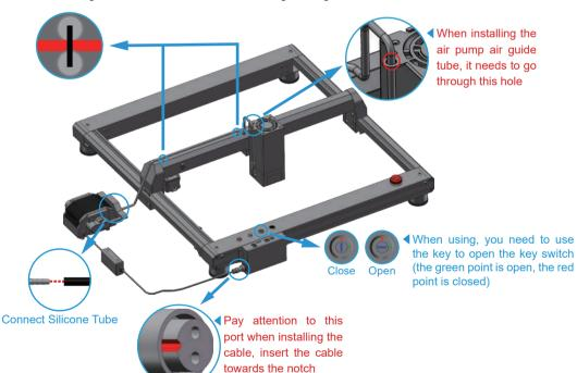
Tip: After the motor cables are connected, please manually move the X or Y axes slowly and DO NOT manually move the axes quickly , otherwise it will cause damage to the motherboard
