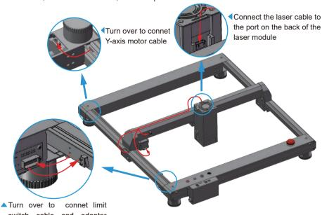
switch cable and adapter board terminal cable, The marked line of the terminal on the adapter board faces up
