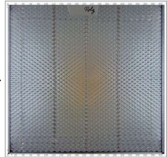
Camera overlay after alignment calibration, the honeycomb appears square and centered within the work area.
