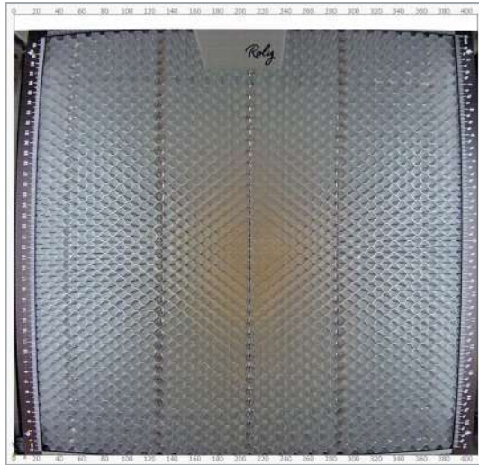
Raw camera image. Note the edges of the honeycomb are bowed outward. If this is what you see, import the camera settings file before proceeding further.
