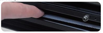
Adjust Belt Tightness: Slowly and Gradually (Half a Turn Each Time) Rotate the Belt Adjusting Screw In the Positive Direction Until It Reaches the Proper Tightness.
