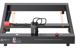
• If One Y Axis Has Reached the Limit Position but Another Y Axis Has Not, You Need to Adjust as Follows: Loosen the Coupling, Manually Move the X Axis to the Correct Limit Switch Position, and Re-tighten the Coupling.
