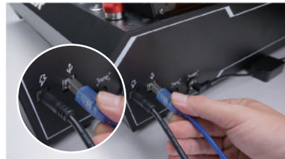
Step 2: Connect the USB cable.
