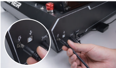
Step 1: Connect the power cord.
