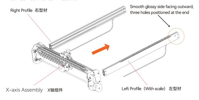
Note that the belts of the left profile and the right profile **ge** oriented downwards! 注意左型材、右型材的皮带方向朝下!
