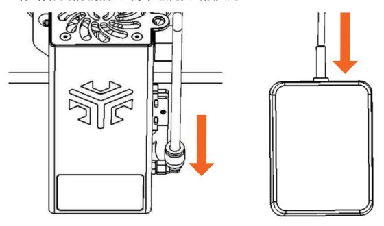
9.2 Connect the adapter, engraving machine and air pump as shown the figure by using two power cables.
