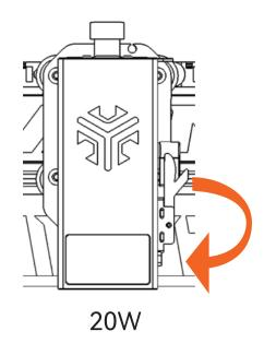
Rotate the nut by hand to make the focusing column contact with the board 旋转手拧螺母使调焦柱与木板接触
