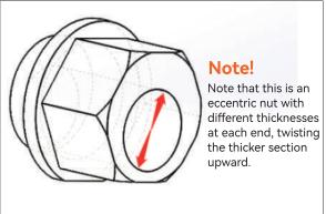
Note: Before pushing the X-axis assembly into the Y-axis section bar, it is necessary to adjust the eccentric wheel to increase the spacing between the pulleys on both sides, to avoid damaging the pulley due to the too close spacing between the pulleys during installation
