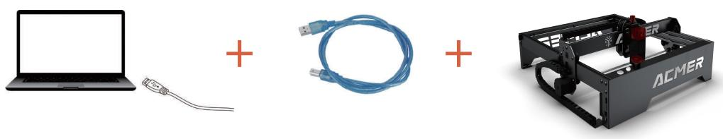
2. Open LaserGRBL software and select the correct port number and baud rate: software-115200
