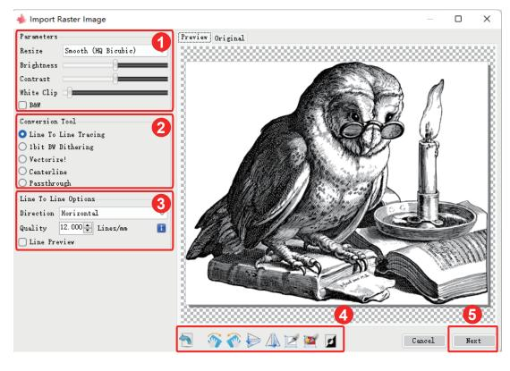
LaserGRBL can adjust the brightness, contrast, and other attributes of the target image. When the parameters are adjusted, you can see the actual effect in the preview window on the right and can try to adjust it to what you think is satisfactory.
