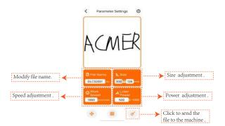
Tips: Before sending files to the machine, make sure there is a memory card on the motherboard
